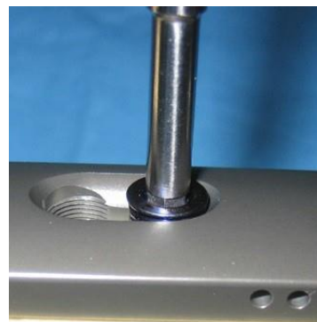
Insert locking screw.
