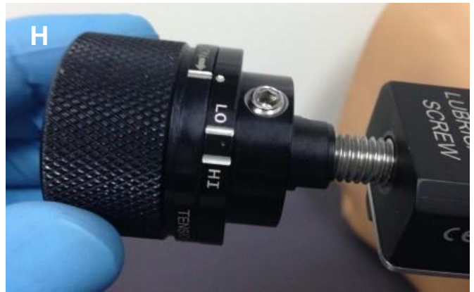
Confirm zero alignment of knobs prior to tensioning.
