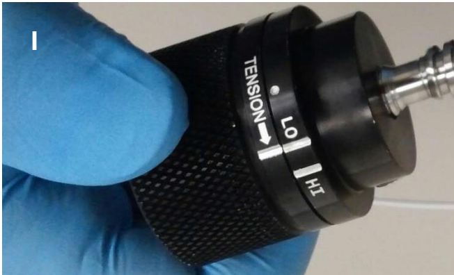
1 st mark indicates 80 lbs (360 N) compressive force.
