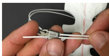
B. Feed cable strands through locking clasp.
