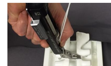
G. Hold cable strands over cleats with thumb or finger and begin to tension cable by turning knob clockwise.
