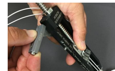
I. Pull back on lever until it stops to fully seat locking wedge.
